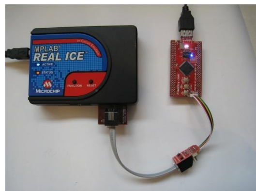
Figure 2: Connecting the Microchip REAL ICE debugger with the PIC32-PLUG-IN-DEV
